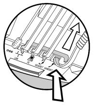
**2.** On the back of the phone, remove the key located behind the hook switch and reposition it so that the end tab (at a 45<sup>0</sup> angle) is facing up.
