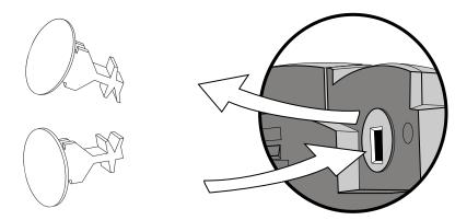
**3.** With mounting tab of the base unit facing up, fasten the base unit to the wall mount using wall anchors (not included).
