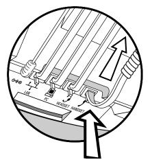
**2.** Align the two protrusions on the bracket with their corresponding holes in the phone.
